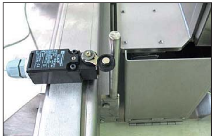
Picture 3: end run interrupter to invert direction and count cycles.
